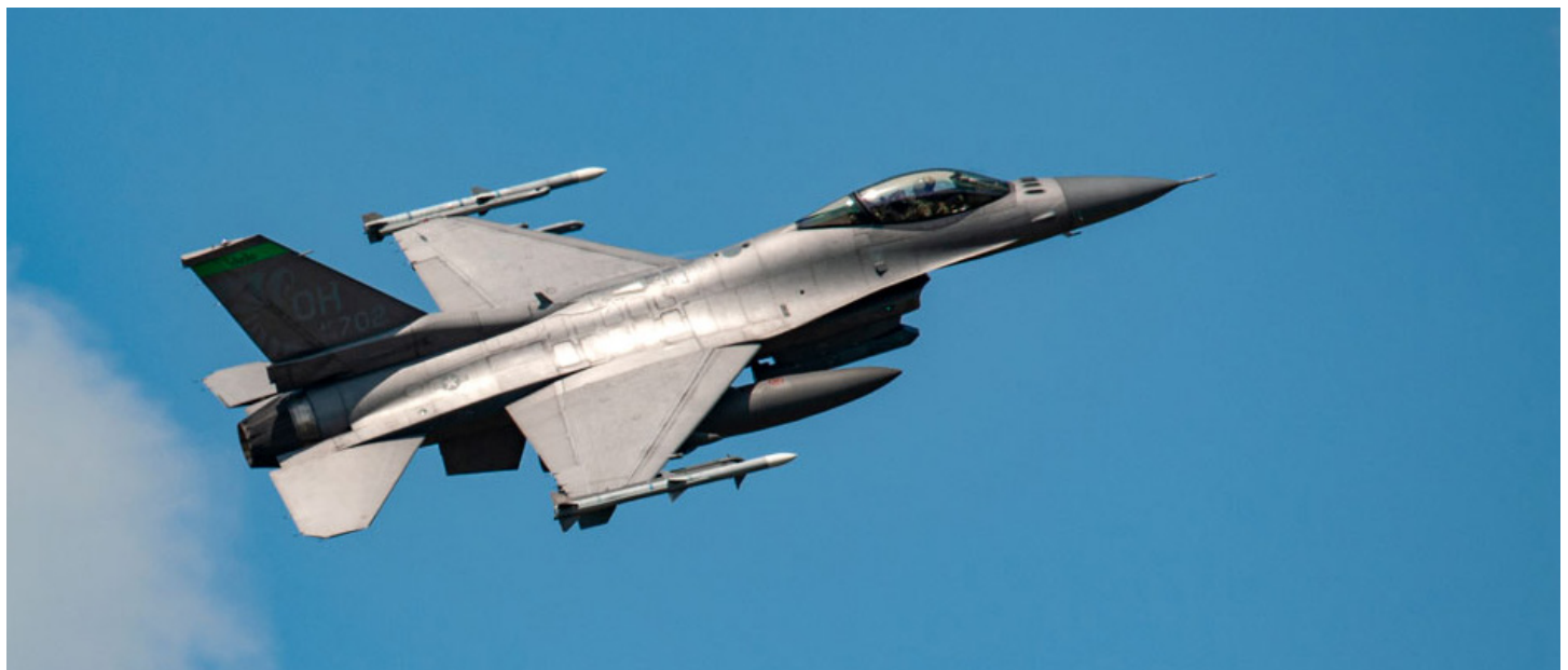
A U.S. Air Force F-16 Fighting Falcons assigned to the OH National Guard's 180 th Fighter Wing, takes off for a training mission, in Swanton, OH. Flying the Lockheed Martin F-16CM Fighting Falcon, a multi-role fighter aircraft with Pratt and Whitney F100-PW-229 engines, the 180FW has access to military operating airspace and air-to-ground gunnery ranges suited for the capabilities of the F-16. The Alpena Airspace Complex, MI, and Buckeye Airspace, OH, are supersonic, chaff/flare capable with full radar ground control intercept and Link-16 capable.
