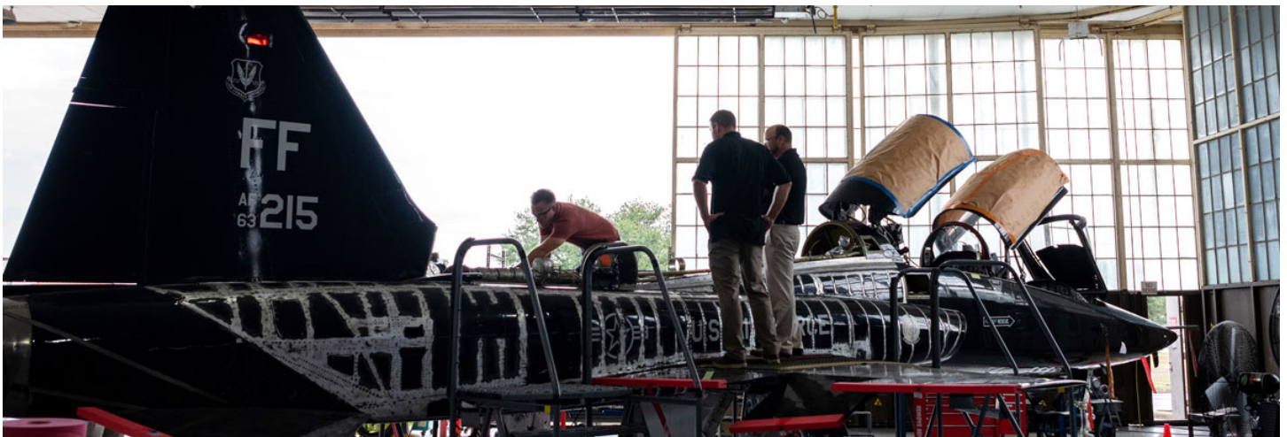
Zach Burleson (left), 809 th Aircraft Maintenance Squadron, Non-Destructive Inspection technician, works on a T-38 as part of the Talon Repair Inspections and Maintenance (TRIM) program as Larry Hall (center), 809AMXS, and Robert Pilarczyk (right), Hill Engineering observe at Joint Base San Antonio-Randolph, TX. The TRIM program will be performed on 190 T-38 aircraft. The capability allows for localized depot-level maintenance to replace or repair key parts.
